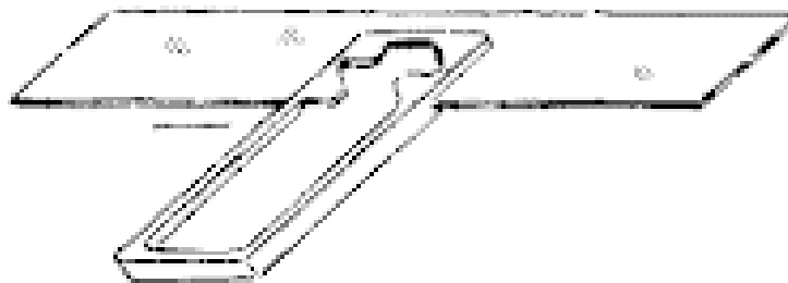
Fig.14 Marking and testing mitre joints
